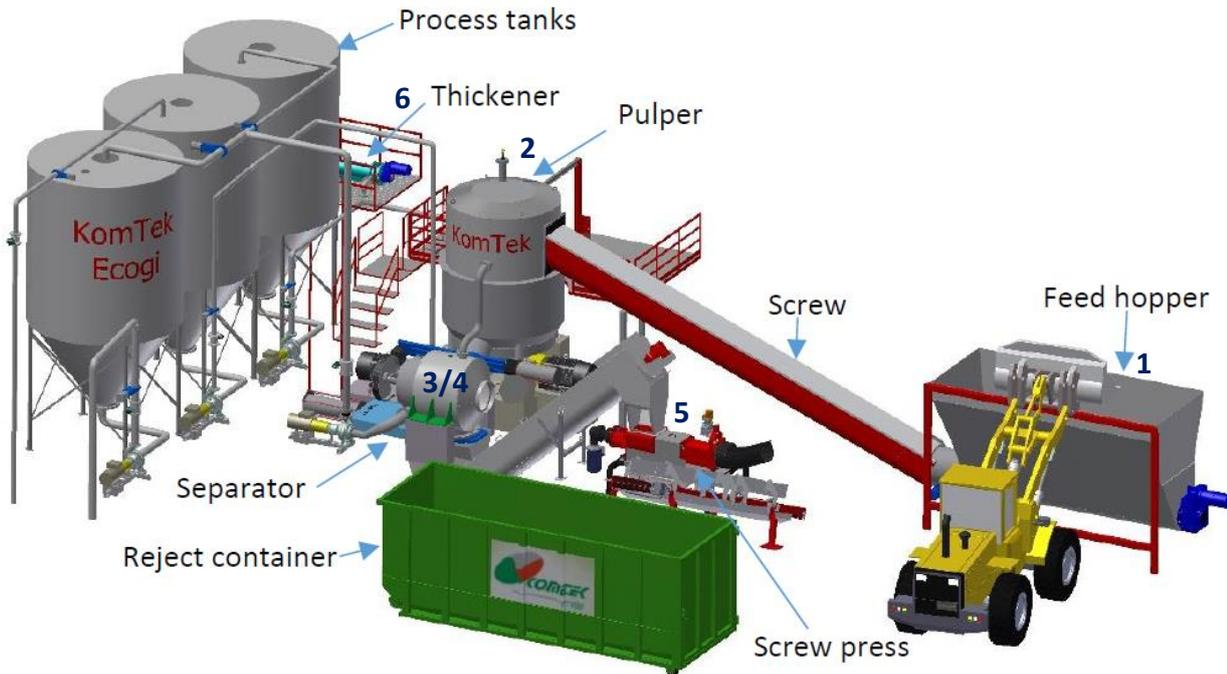
The Ecogi technology has been developed for source-segregated organic waste from households and commercial enterprises. The system is designed with robust components to cope with the challenges in this kind of waste. The numbers below refer to the flow diagramme in figure 1.
