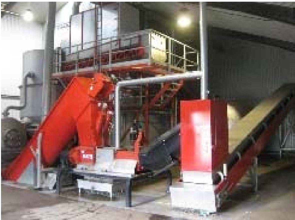
Most would agree that removing physical contamination is best done prior to AD processing i.e. during feedstock pre-treatment. Once removed contamination ceases to put at risk equipment downstream and ensures the final purity of digestate.
